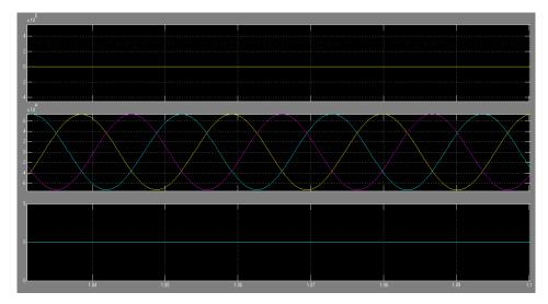
Fig. 6: Alternator 02; (a) Relay status, (b) 3 phase voltage, and (c) 3 phase current.
