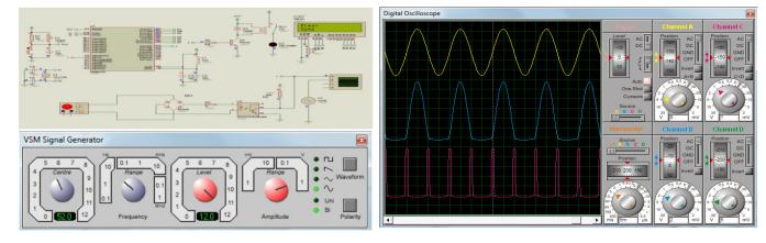
Sinusoidal signal, Pulsating DC signal, and Zero crossing Puls
