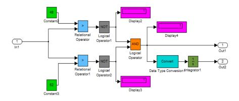
Fig. 2: Over and under frequency detection block on SIMULINK.
