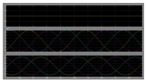
Fig. 3: Alternator 01, 02 & 03; (a) Relay status; (b) 3 phase voltage, and (c) 3 phase current.
