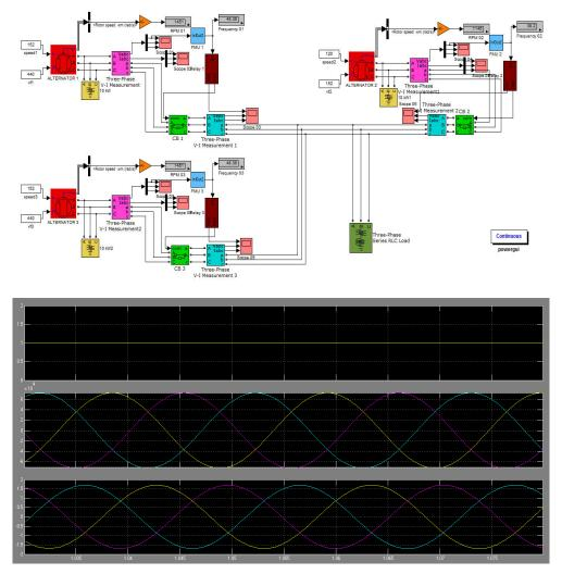
Fig. 5: Alternator 01 & 03; (a) Relay status, (b) 3 phase voltage, and (c) 3 phase current.
