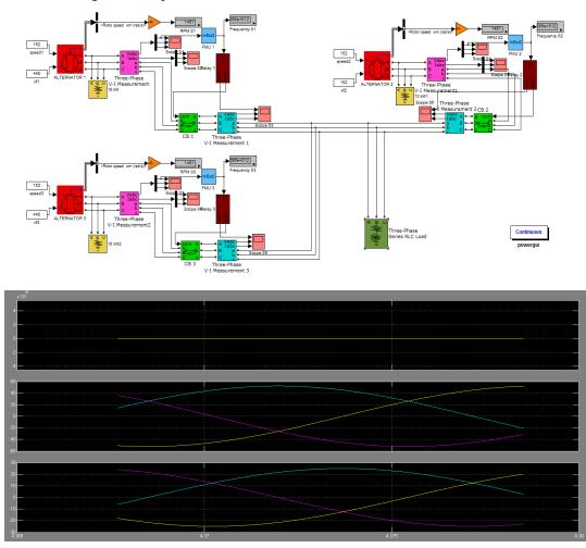
Fig. 8: Alternator 01, 02 & 03; (a) Relay status, (b) 3 phase voltage, and (c) 3 phase current.
